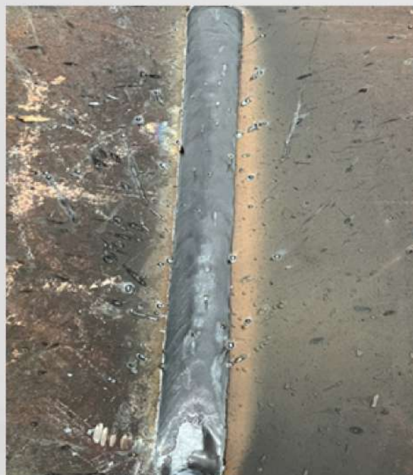
Test weld seam(base+fill+cover, solid core welding wire)
