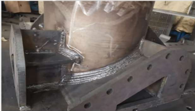
Multi layer and multi pass welding of fillet welds with inner and outer corners
