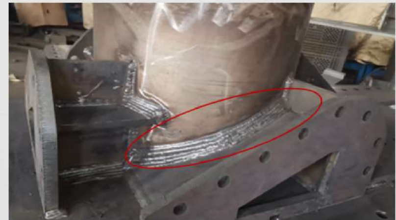
Multi layer and multi pass welding of intersecting line welds with a 30 degree climbing slope
