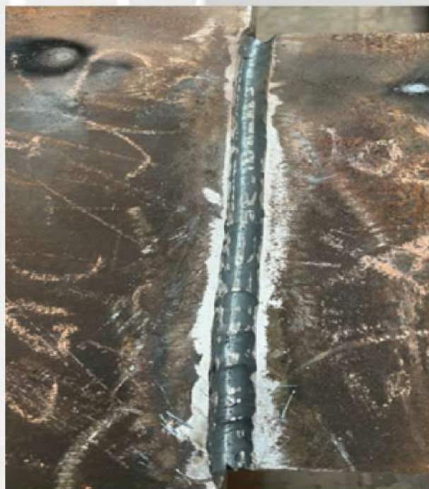
Groove weld seam (air gouging+manual polishing)
